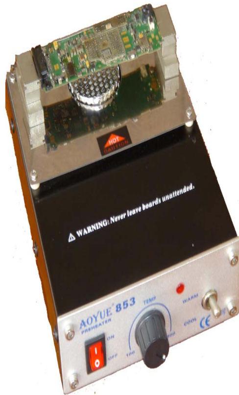
Compact preheating device preventing panel board distortion.
